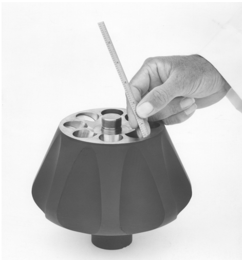
Figure 3 Measuring Distance from Cap to Rotor Tray
